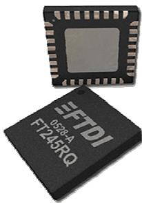
The middle of the part has a metal contact pad – like most QFN packaged parts. It may be there for grounding or heat conduction, depending on the specific part. The float that I'm talking about happens when we lay too much solder paste on the PCB for that center pad.
