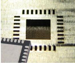
This is what a just about worst-case stencil would look like. Actual size for this part is 7 x 7 mm. Note how much surface area that the center pad has compared to the row of side cutouts. With most SMT components, it is standard procedure to reduce the size of the paste cutout area in the stencil. In a case like this, it is difficult to reduce it enough and still get even paste distribution. The proper option is to segment to solder stencil area.
